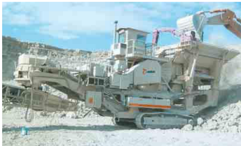
Mobile primary crushing for cement plant in the USA using LT140 + LL12.
