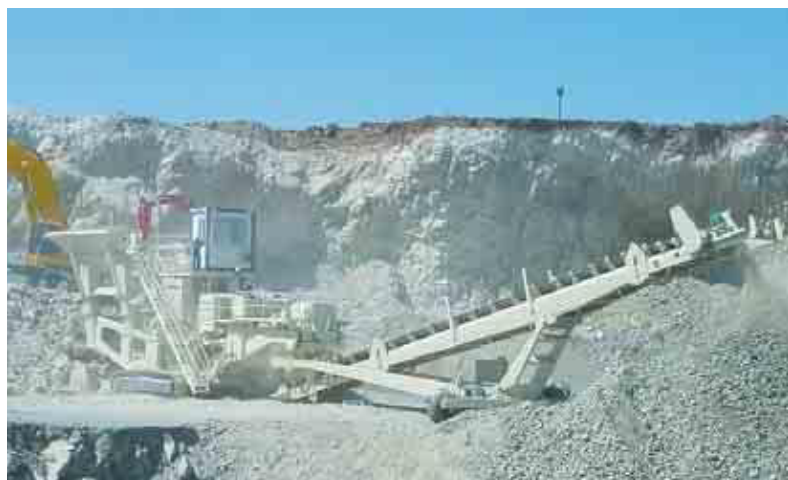
A mobile quarry application in Spain with a primary crushing plant LT140 and a TRLP12-20 conveyor.
